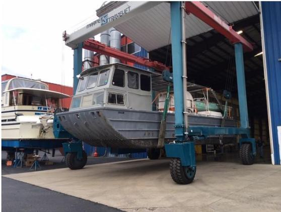
This is a photo of the craft used by the team from SU-SUNY ES&F last July to perform seismic profiling of the sediments beneath Oneida Lake.
